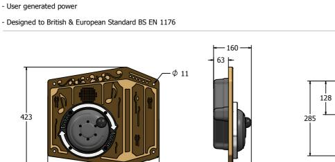
Mounting Cutout & Fixing Holes 320 Ø 11 320 253 142 420
